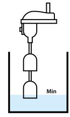
And, the pump stops at the minimum level.
