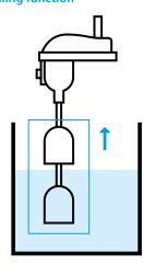
As the water level encounters the (max level) float the combined float unit starts to lift.
