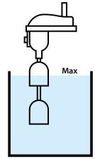
As the combined float unit lifts the magnetic switch closes. The pump then starts and the tank begins to empty.
