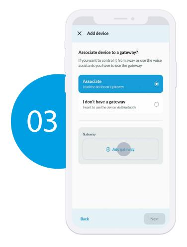
Select "Add gateway" if you wish to use a Type 1Y.GU.005.1 gateway to access the system remotely and/or with voice assistants, then follow the pairing procedure.
