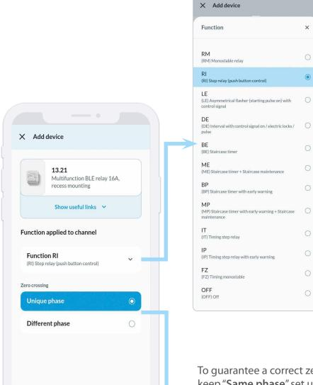
A large selection of functions become available, such as step relay (push-button or switch), staircase light timer, flashers, pulses (DE 2 sec) and many more. Select "More info" for further information and the related timing diagrams.
