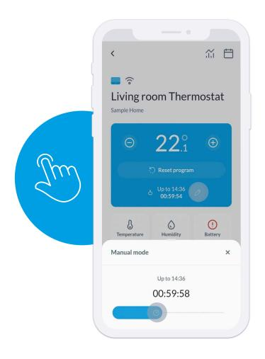
When you press + or – from the thermostat home screen, the desired temperature is mantained for a hour.
