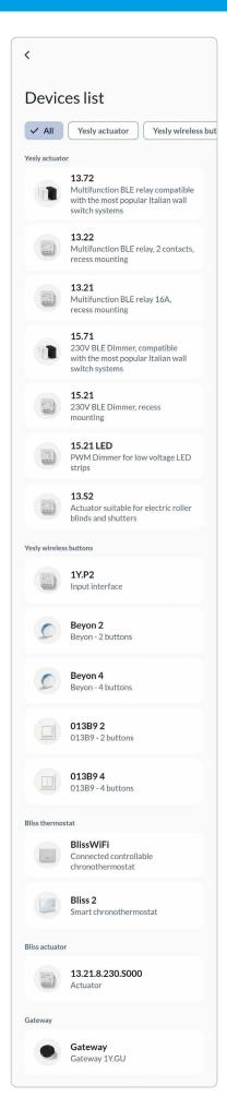
After selecting on "Add Device", the Device Catalogue is displayed, from which the user can select the product to be installed in the electrical system later on. It's possible to choose from the YESLY and BLISS devices that can be configured through the Finder YOU App. It is strongly recommended to do the "logic" configuration of the system first and then to apply the settings to the devices once installed and powered up.
