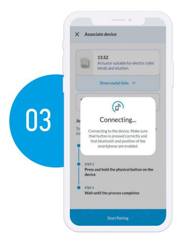
Keep the physical button on the device pressed (either P1 or P2) or bring and maintain voltage on the terminal; by other means (keeping safety as a priority).
