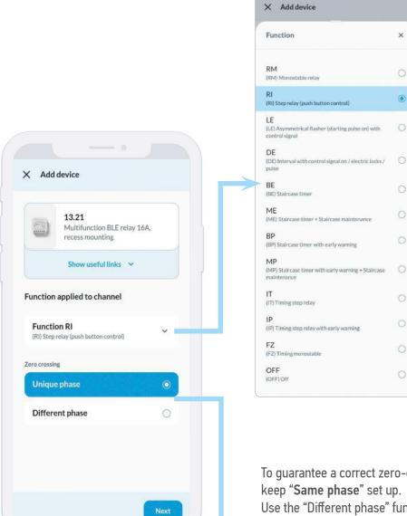
A large selection of functions become available, such as step relay (push-button or switch), staircase light timer, flashers, pulses (DE 2 sec) and many more. Select "More info" for further information and the related timing diagrams.
