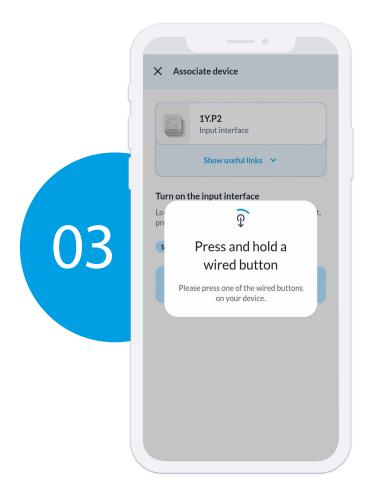
Once the desired input interface is selected, keep the physical button on the device pressed (either P1 or P2) or bring and maintain voltage on the terminal by other means (keeping safety as a priority).
