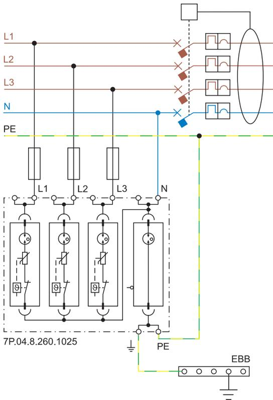
Schéma de raccordement "V-shape" (fusible max = 125A)
