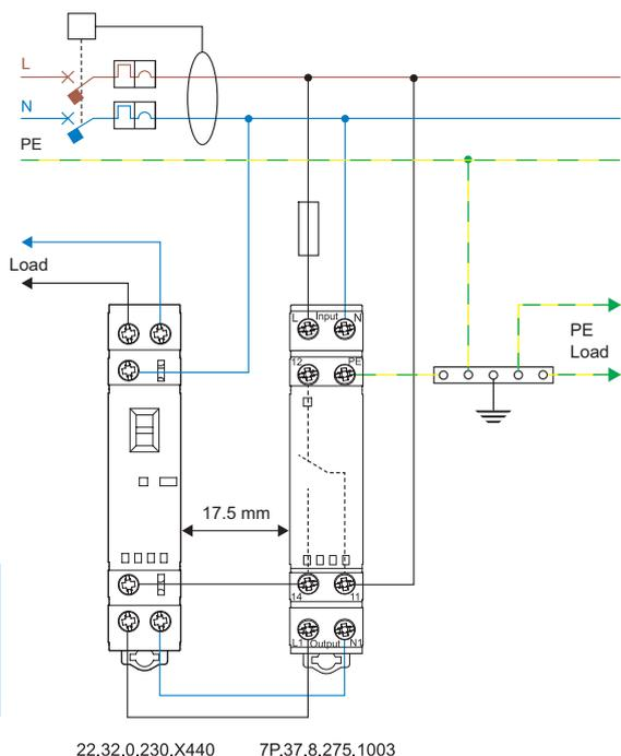
TTT, TN-S MONOPHASÉ EN AVAL DU DIFFÉRENTIEL : RACCORDEMENT SÉRIE + BUS
