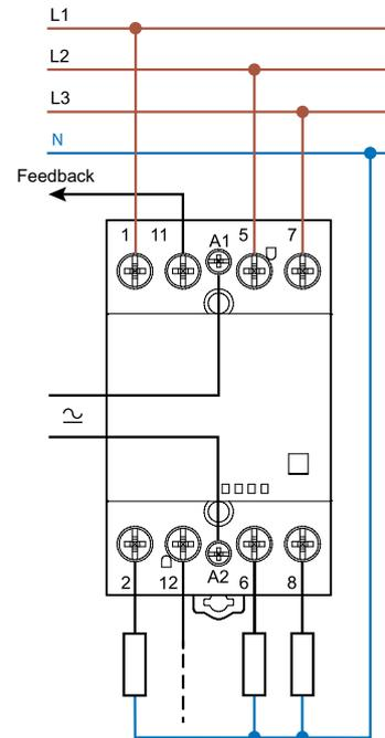
Example of application of contactor with Mirror Contacts: Normally closed contact is definitely in open position if the normally open contact is closed
