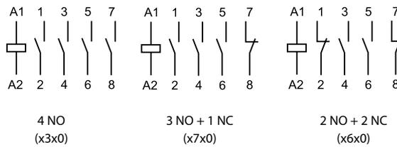
\* Contact gap  $\geq 3$  mm for NO contacts only;
