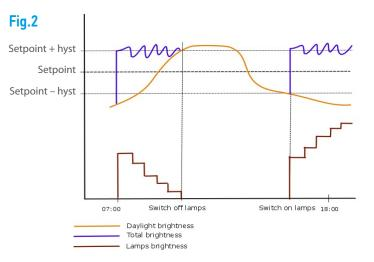
Starting from 7:00 AM, the device constantly detects the presence condition. Since at that moment the natural brightness is lower than the setpoint – hysteresis, it evaluates through the curve constructed with the calibration how much artificial brightness is necessary so that the total brightness is mantained around the setpoint value + hysteresis and turns on the lights, for example with the percentages OUT1 = 30 %, OUT4 = 20%.
