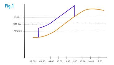
Starting from 7:40 AM the device constantly detects the presence condition (movement).
