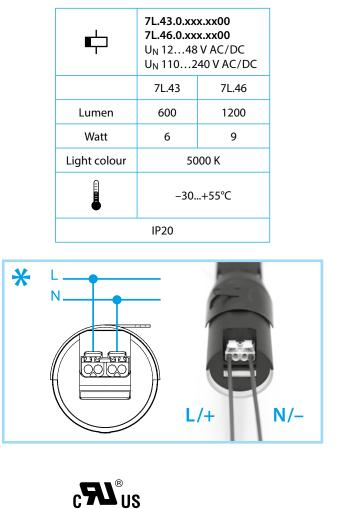
For Canadian market, in the end-use the devices shall be connected to a Surge-Protective device, Type 1 or 2 or 3, rated minimum 240 V and with a maximum Voltage Protection Rating (VPR) of 2500 Vpk for 7L.4x.0.230.xxxx, rated minimum 50 V and with a VPR 800 Vpk for 7L.4x.0.024.xxxx
