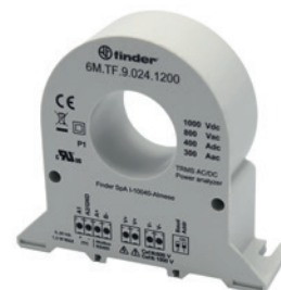
Type 6M.TF.9.024.1200 300 A - 800 V AC, 400 A - 1000 V DC
