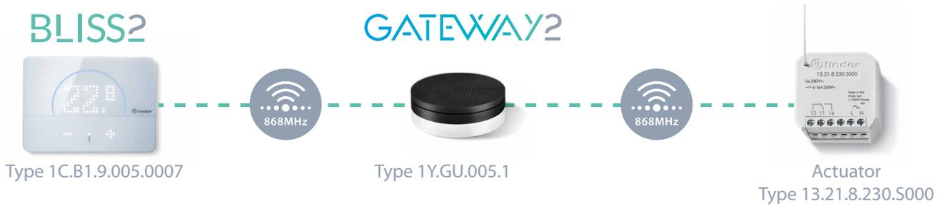
A maximum of 5 actuators can be associated with a single Bliss2.
