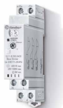
15.11 "Slave" dimmer 1-10 V input, driven by 15.10 or by other 0-10 V/1-10 V output devices Maximum lamp load 400 W
