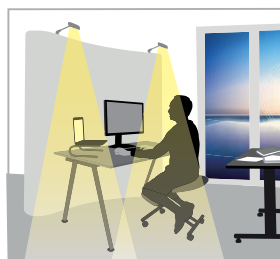
Model 18.51 automatically switches the lights on when the light level is low and movement is detected.
