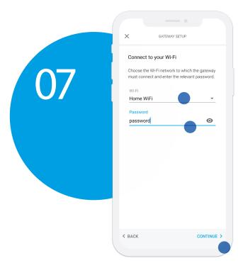
Select the network to link the device with, then insert the password. Press on 'CONTINUE' to go on.
