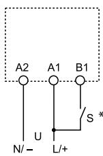
\* With DC supply, positive polarity has to be connected to terminal B1, terminal (according to EN 60204-1).
