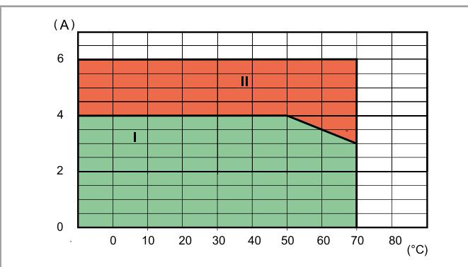
I: SSR installed as a group (without gap between sockets)
