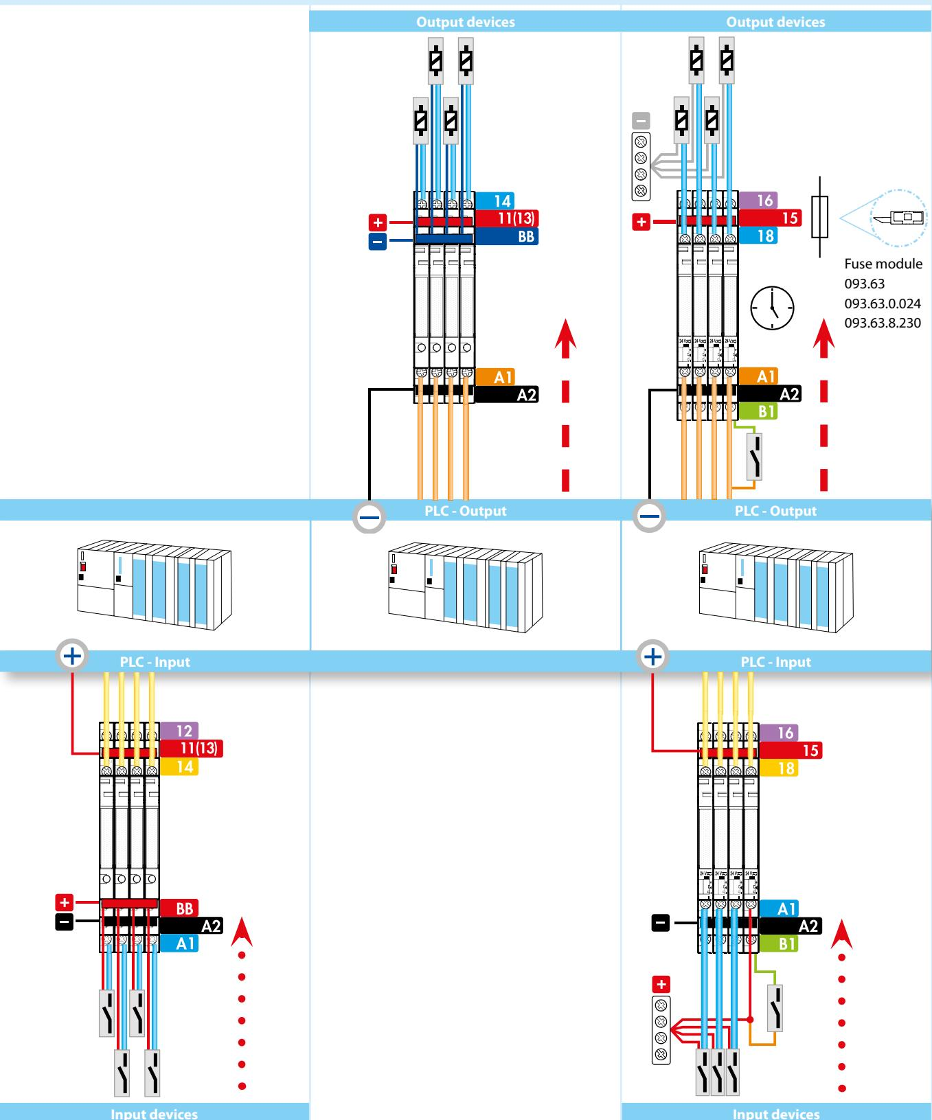
**MasterBASIC - EMR****1 Pole interface module, 6.2 mm wide, ideal for PLC and electronic systems**
