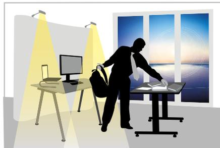
With low light and movement/presence detected the 18.51 switches the lamps On automatically.
