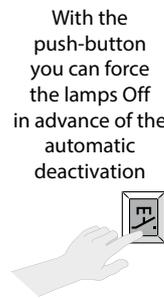
With the push-button you can force the lamps Off in advance of the automatic deactivation
